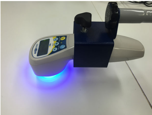
Figure 1. The 465 nm blue light therapeutic device (MR4 ACTiVet PRO™ device, Multi Radiance Medical®; Solon, OH, USA) irradiating a 35 mm petri dish containing tryptic soy agar plated with a bacterial isolate.
